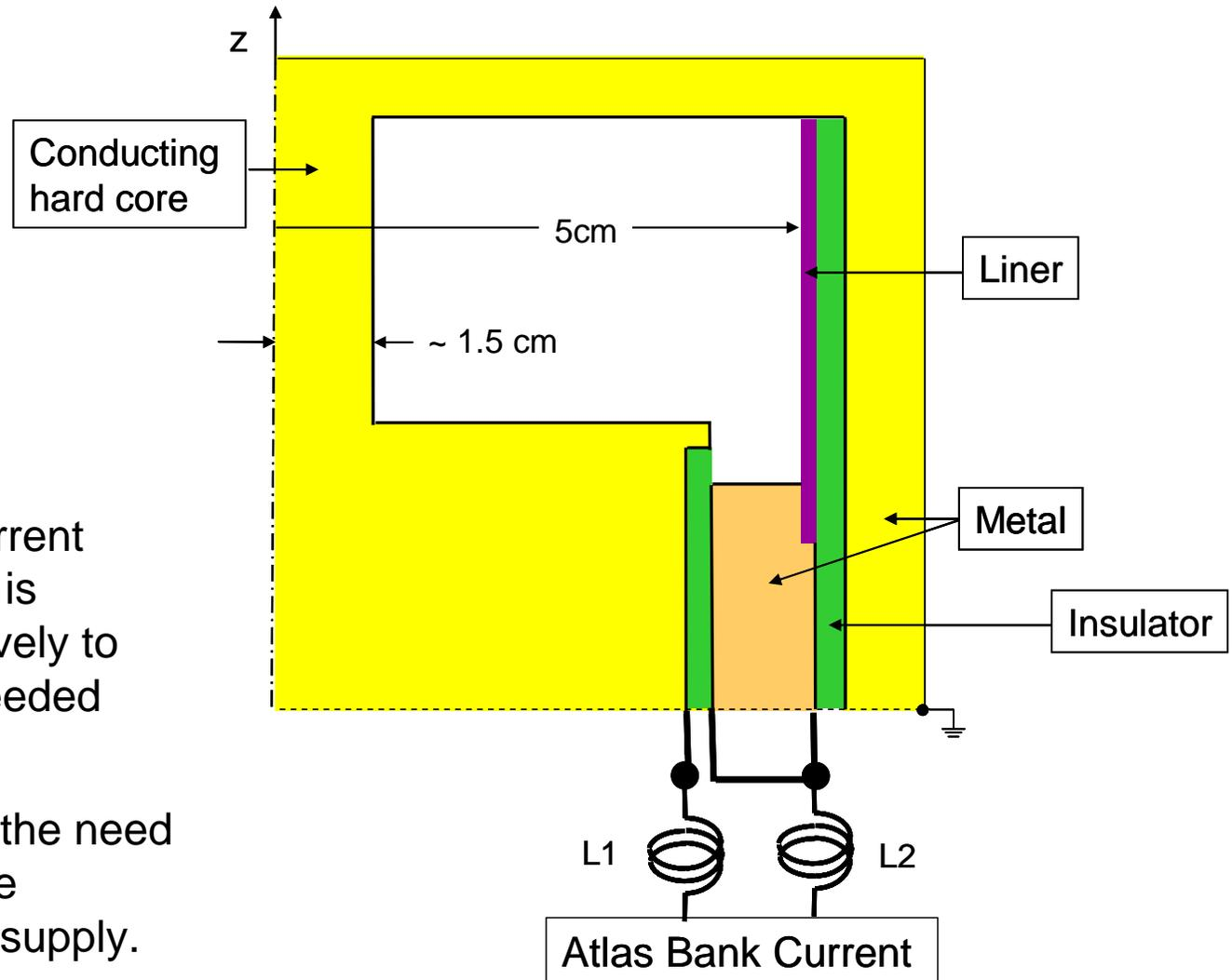
Part of Atlas current driving the liner is diverted inductively to generate the needed initial flux
