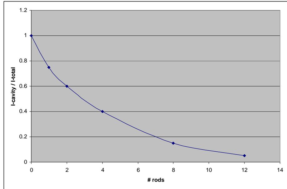
Data prove that inductive divider is readily constructed to give desired current of  $\sim 1/8$  total.
