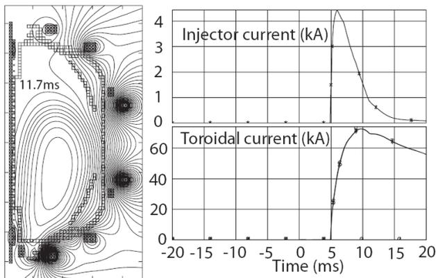
Figure 2: Shown are the poloidal flux contours, injector current and CHI produced toroidal current for NSTX discharge 118340 [Ref. 17].
